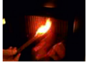
Illustr. 1: Chimney draught test
